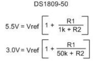
Using the above equation, we choose the  $50k\Omega$  pot for a wider voltage range. We determine that R1 is  $119.5k\Omega$  and R2 is  $33.6k\Omega$ . The 2.5V range allows for 39mV/step accuracy.
